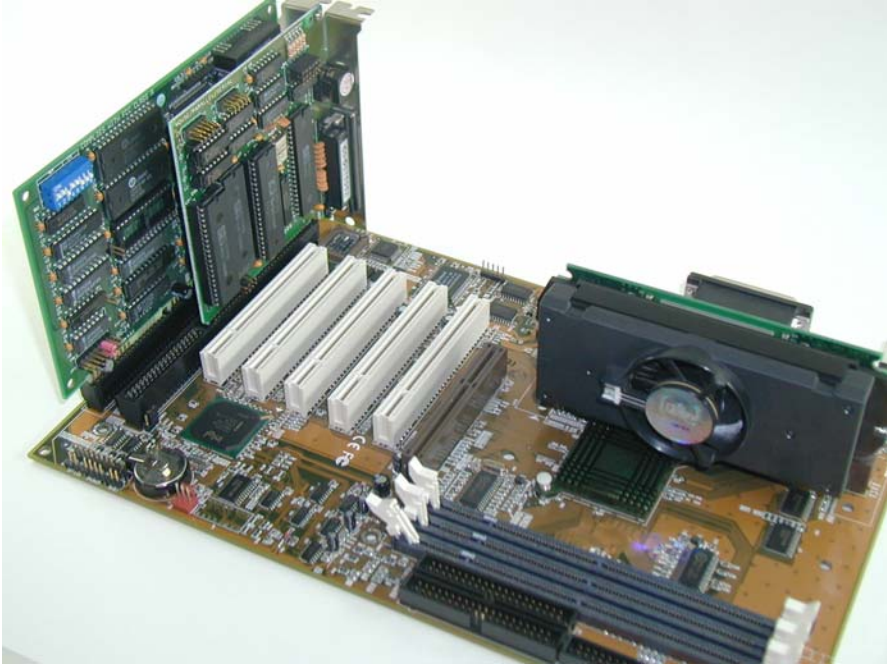
Fig. 6.1 Modular hardware implementing a PC.
